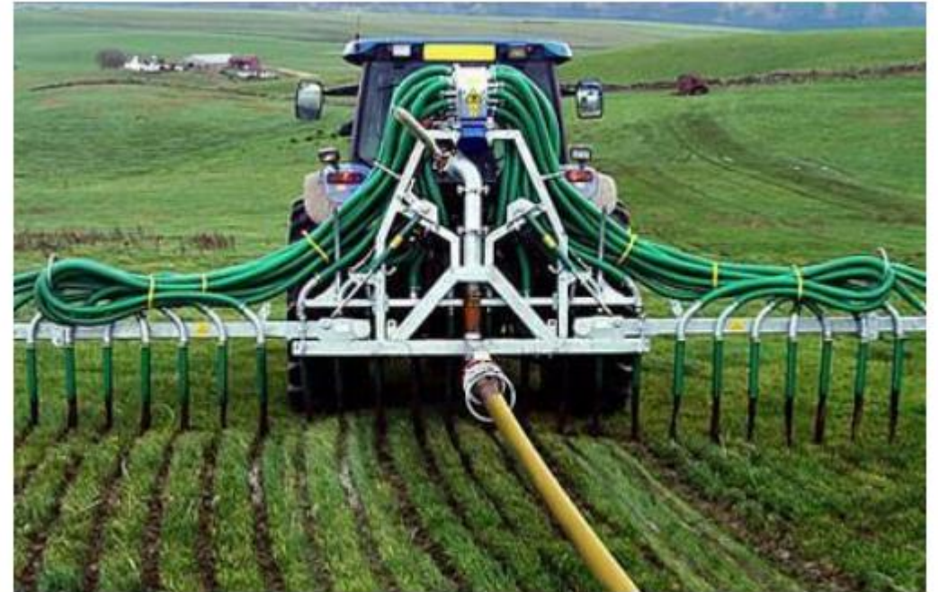
Image: Slurry spreading with dribble bars using an Umbiblical system
