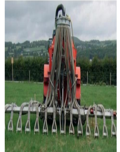
Conventional Splash Plate Method vs Low-emission Trailing Shoe Method
