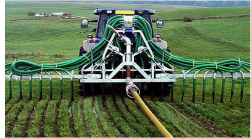
Image: Slurry spreading with dribble bars using an Umbiblical system Source: Slurrykat
