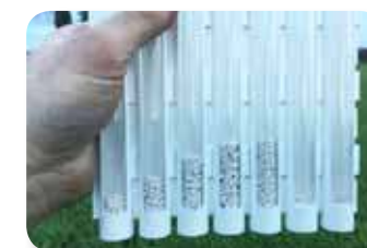
Figure 8:- Fertiliser spread pattern where boundary mechanism not in place
