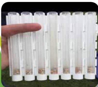
Figure 7:- Collecting tubes show spread pattern from tray test and evenness of fertiliser application.
