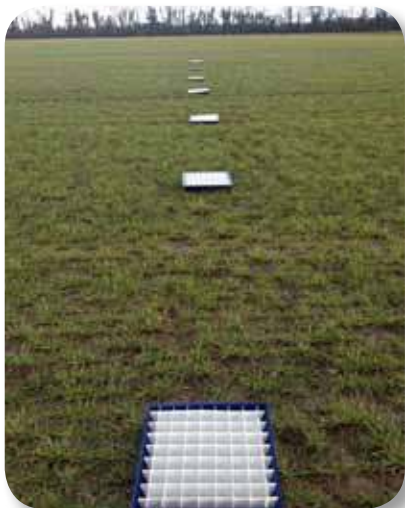
Figure 5:- Tray testing during the season can reveal exactly how fertiliser is being applied. Place trays every 2 to 3 metres across the spread to get a measure of spread pattern.
